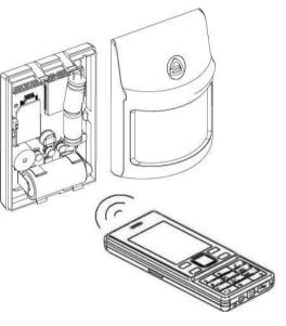
In 30 seconds after turning on, use your mobile phone SMS feature to send your mobile phone number to the motion detector SIM card. Use the following number format: 1)+XXXXXXXXXXXX, where "1)" is the index number for the first phone number to be registered (maximum 6 phone numbers allowed)
