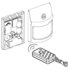
When you finish programing the motion detector using your mobile phone you have 30 seconds to press the remote controller button. This will register the controller with the motion detector
