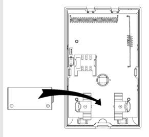
Insert the battery into the battery holder in the motion detector, observing polarity.
