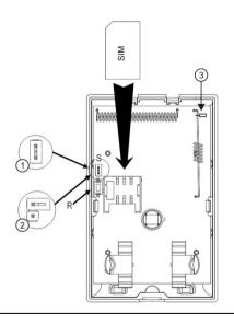
Insert the SIM card into the SIM card holder the way it's showed on the left picture. Set the jumper to position 1 or position 2.
