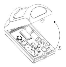
1. Lift up and remove the motion detector lid.
