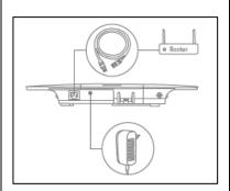
First connect the LAN cable provided on the underside of the Smartvest and connect this to your router,
