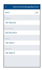
The Smartvest is set to DHCP by default. This means that the Smartvest is automatically assigned an IP address, subnet mask, gateway and DNS server by your router.
